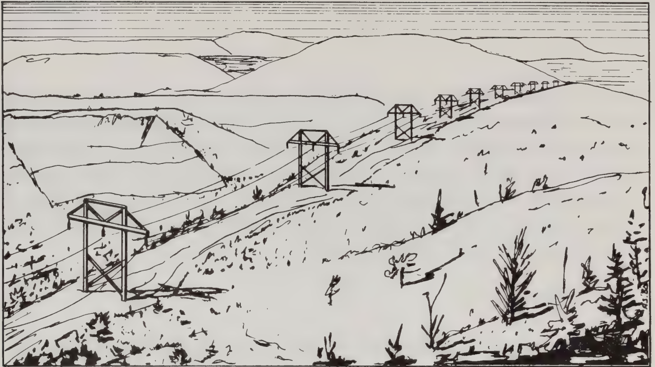
Poor Location & Excess Clearing
